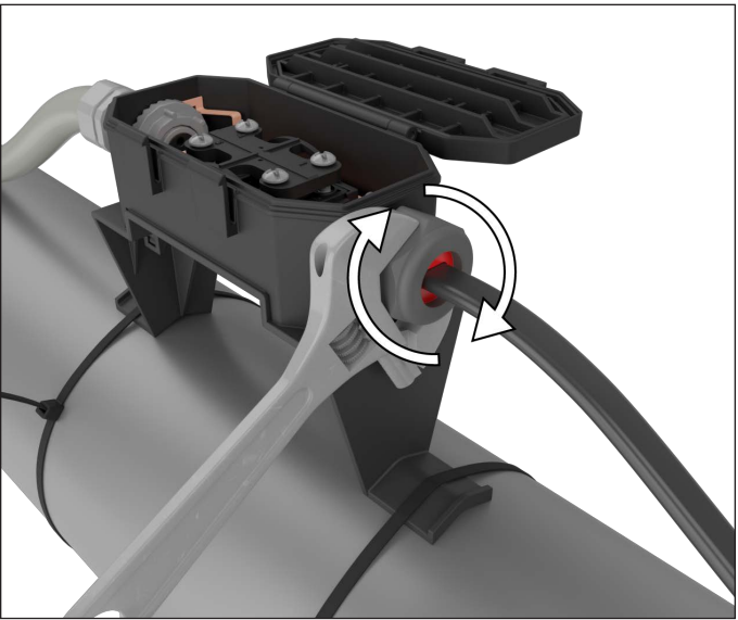
8. Torque gland nut (8 Nm for "LINK-B" version, 5 Nm for "LINK-D" version) to seal around cable.
